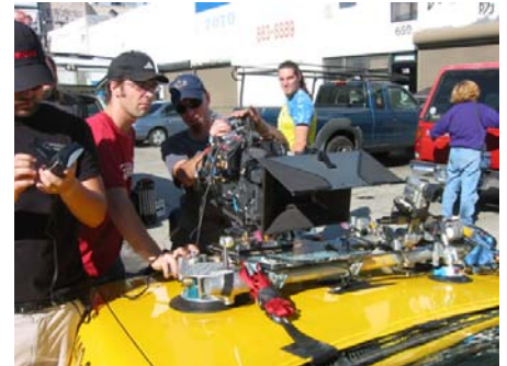
The crew rigging a hood mount.
